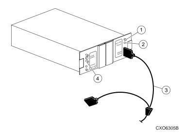
Figure 1–9. ECB for Dual-Redundant Controller Configurations
